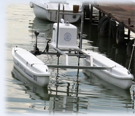
Functional model of autonomus utilitarian naval platforms
